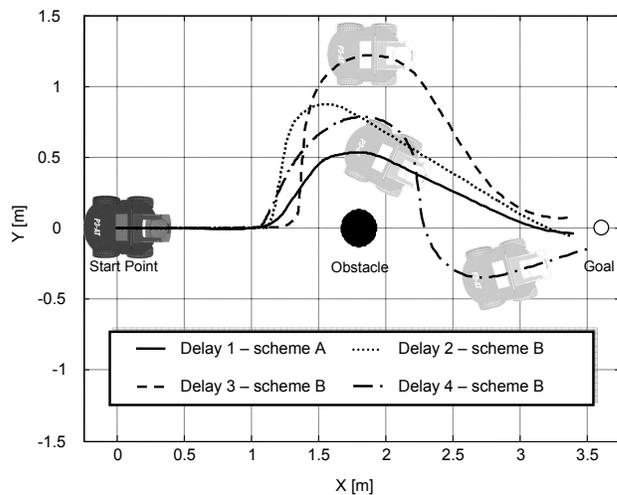
Fig. 11. Trajectories followed by the remote mobile robot using the scheme B.
