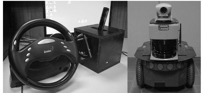
Fig. 9. Mobile robot teleoperated through a joystick with force feedback and steering wheel.
