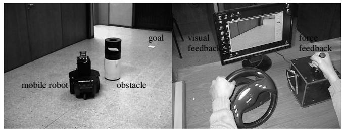
Fig. 15. Image of the teleoperation experiment carried out.
