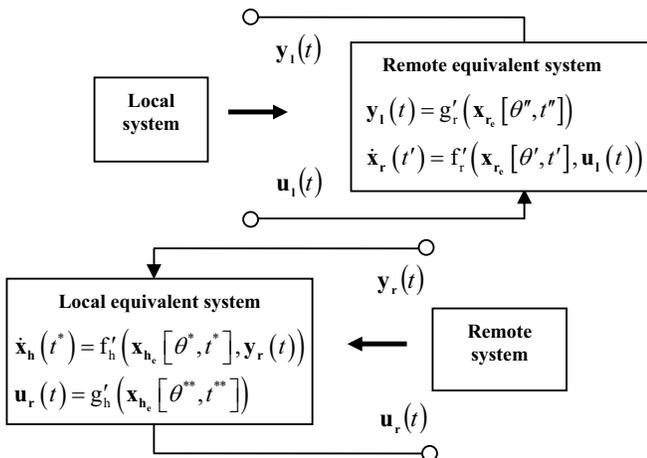
Fig. 3. Local and remote equivalent systems.
