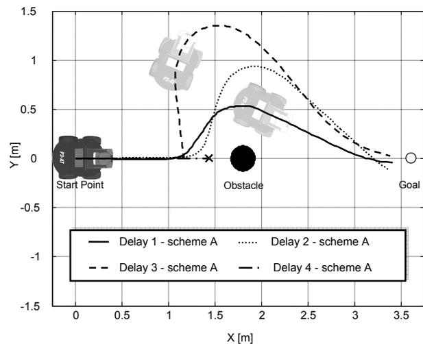
Fig. 10. Trajectories followed by the remote mobile robot using the scheme A.
