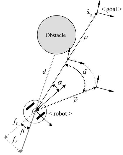
Fig. 8. Repulsive force and distance and angular errors.
