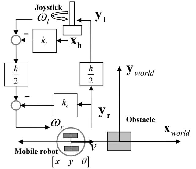
Fig. 6. Teleoperation system of a mobile robot with force feedback.
