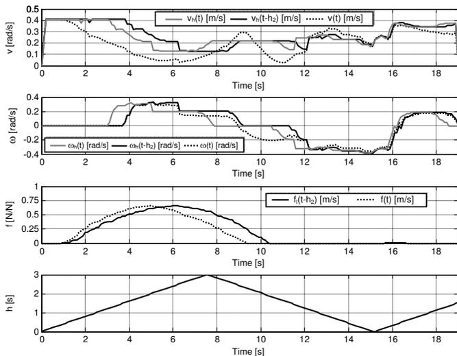
Fig. 14. Linear and angular velocity commands and real velocities for a delay-type 4 using scheme D.
