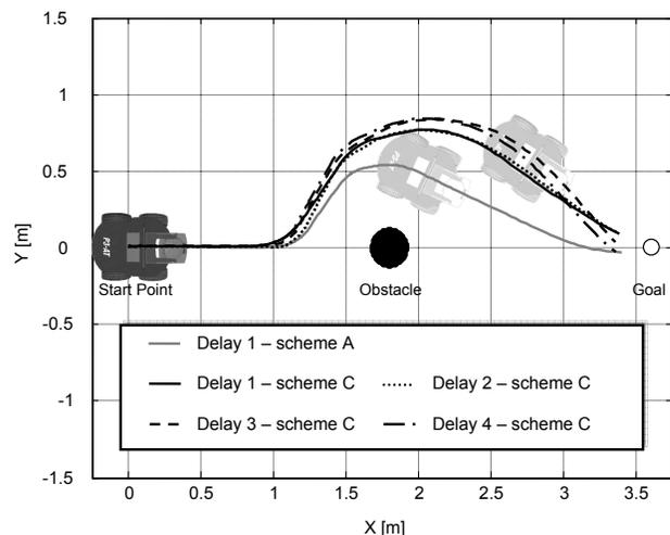
Fig. 12. Trajectories followed by the remote mobile robot using the scheme C.
