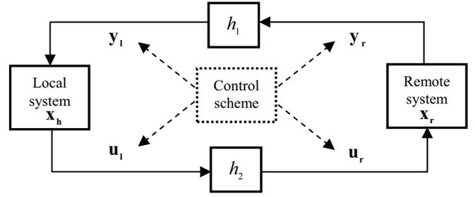
Fig. 2. Control scheme applied to teleoperation systems.
