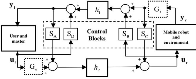
Fig. 7. General control schemes for bilateral teleoperation of mobile robots.
