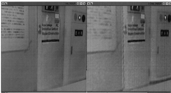
Fig. 17. Comparative result of virtual viewpoint image created from the generated 3-D model and textures (left: high-resolution texture, right: single input texture).
