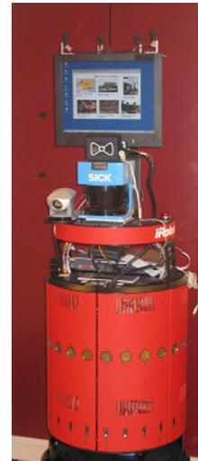
Figure 1. The B21R combines audio and visual interfaces
