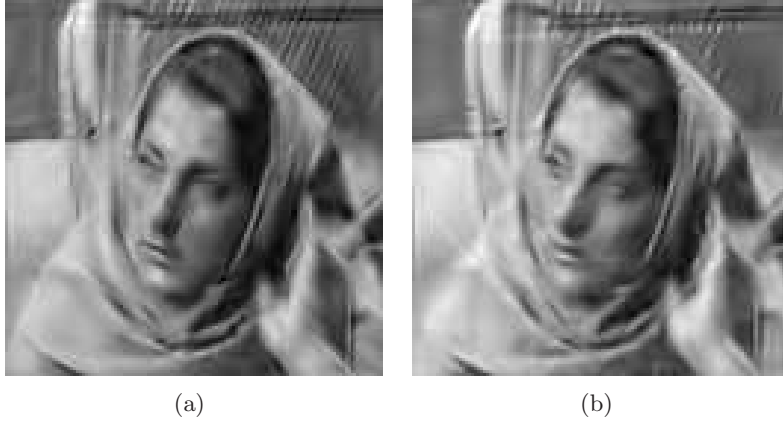
Figure 2: 300 atoms reconstruction results. (a) dMP : J = 5 , K = 8 , PSNR: 26.63 dB, 4634s. (b) gMP : J = 3 , K = 4 , \kappa = 10 , PSNR: 26.68 dB, 949s.
