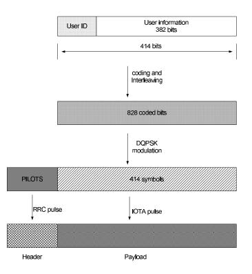
Fig. 1. Signal Structure
