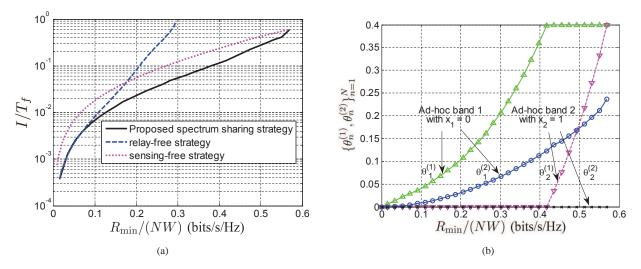
Fig. 4. Simulation results of the proposed frame-level transmission control strategy of the CRN with parameters given in Table I. (a) Normalized average collision time  $(I/T_f)$  versus required uplink spectrum efficiency  $R_{\min}/(NW)$ , (b) optimized transmission time fractions  $\{\theta_n^{(1)}, \theta_n^{(2)}\}_{n=1}^N$  versus required uplink spectrum efficiency  $R_{\min}/(NW)$ .
