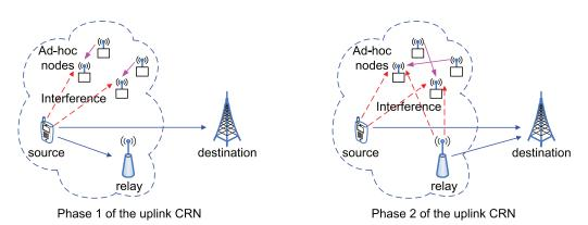
Fig. 1. System model. In Phase 1 (left plot), the source node broadcasts information to the relay and destination, and the transmitted signal interferes with the nearby ad-hoc links; in Phase 2 (right plot), the source and relay transmit signals to the destination simultaneously and both transmitted signals interfere with the ad-hoc links.
