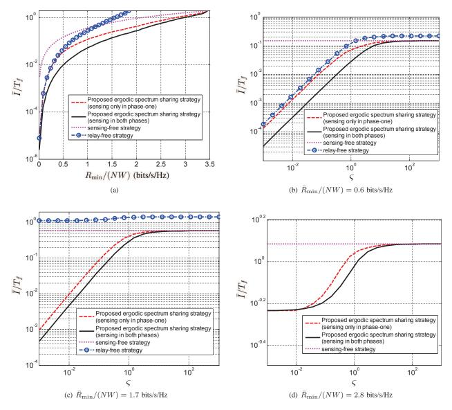
Fig. 6. Simulation results of the proposed ergodic transmission control strategy of the CRN. (a) Normalized long term average collision time  $(\bar{I}/T_f)$  versus required long term average uplink spectrum efficiency  $\bar{R}_{\min}/(NW)$ , (b)-(d)  $\bar{I}/T_f$  versus  $\varsigma$  for  $\lambda = \mu$  and various values of  $\bar{R}_{\min}/(NW)$ .
