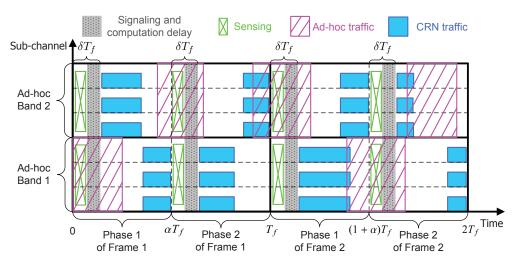
**Fig. 5.** Time-frequency transmission structure by Lemma 2. Here the sensing outcomes of Frame 1 are  $x_1 = 1$ ,  $x_2 = 0$ ,  $y_1 = 0$  and  $y_2 = 1$ , and the the sensing outcomes of Frame 2 are  $x_1 = 0$ ,  $x_2 = 1$ ,  $y_1 = 1$  and  $y_2 = 0$ .
