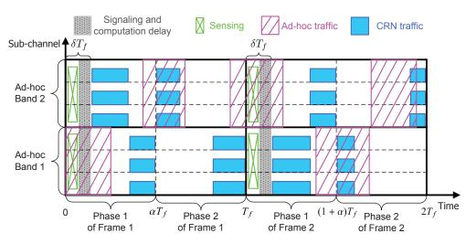
Fig. 3. An example illustrating the spectrum access strategy of Lemma 1. The sensing outcomes of Frame 1 are  $x_1 = 1$  and  $x_2 = 0$ , and the sensing outcomes of Frame 2 are  $x_1 = 0$  and  $x_2 = 1$ .
