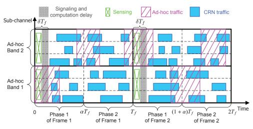
Fig. 2. Time-frequency transmission structure of the CRN and the ad-hoc network. In this figure, the number of CRN sub-channels is 6 (N = 6) and the number of ad-hoc bands is 2 (M = 2).
