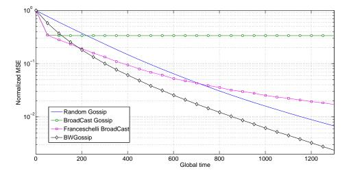
Fig. 1: Mean squared error of the BWGossip and other famous algorithms versus time.
