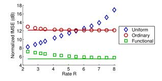
Fig. 5. Empirical and theoretical performance for the uniform, ordinary and functional quantizers for Cauchy  $f_X$  and  $g(x) = e^{-|x|}$ . The distortions are multiplied by  $2^{2R}$  to better indicate the convergence results.
