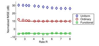
Fig. 6. Empirical and theoretical performance are provided for the uniform, ordinary and functional quantizers for N = 10, exponential  $f_X$ , and  $g(x_1^N) = \min(x_1^N)$ . The distortions are multiplied by  $2^{2R}$  to better indicate the convergence results.
