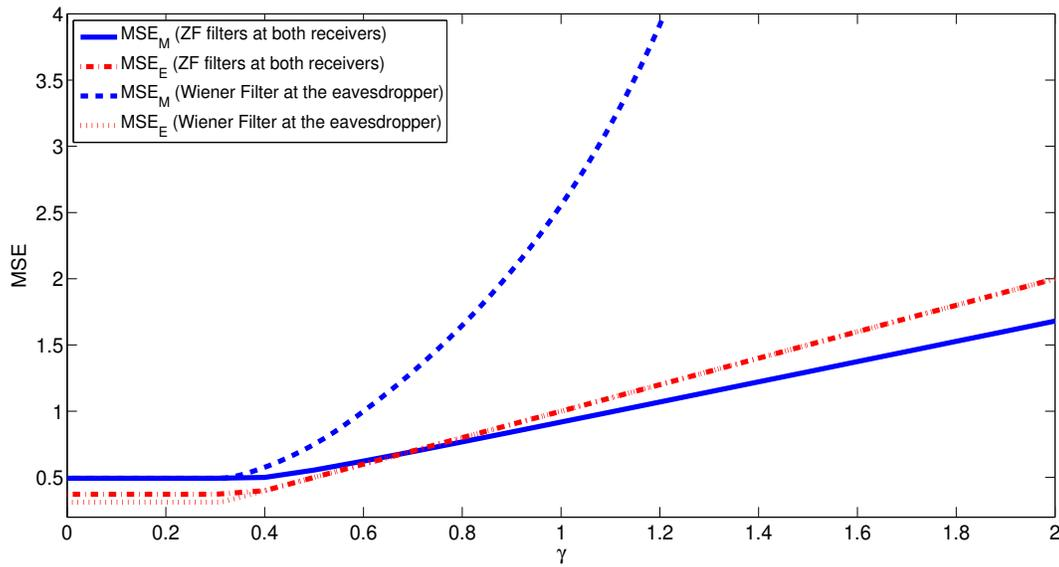
Figure 5. Main and eavesdropper channel MSEs vs. secrecy constraint, for the optimal transmit filter design with ZF filters at both receivers and Wiener filters at the eavesdropper receiver, in a non-degraded scenario ( $P_{avg} = 1$ ).
