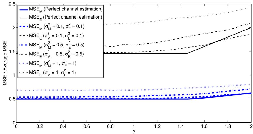
Figure 6. Main and eavesdropper channel average MSEs vs. secrecy constraint, in the presence of channel error estimation, for the optimal transmit filter design with ZF filter at both receivers ( $P_{avg} = 1$ ).
