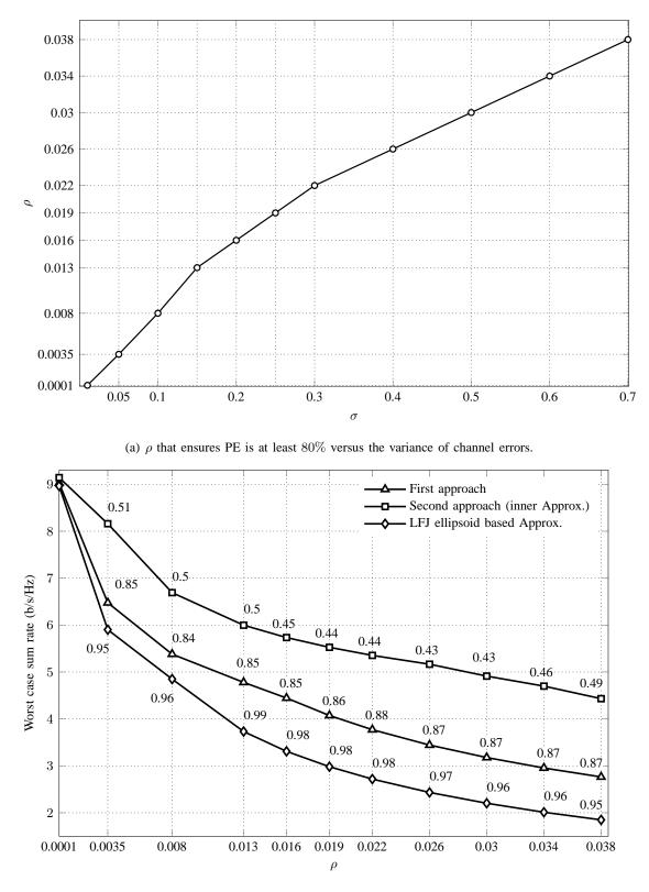
(b) Resulting sum rates versus  $\rho$  obtained from Fig. 7(a). The PEs are shown on top of the marker symbols used for both approaches.
