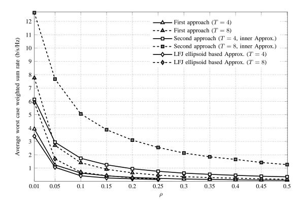
Fig. 4. Average worst case weighted sum rate of proposed robust designs for box uncertainty set with T = 4,8 and SNR = 10 dB. The weights are taken as  $(\alpha_{1,1}, \alpha_{1,2}, \alpha_{2,1}, \alpha_{2,2}) = (1.14, 1.21, 0.52, 0.84)$ .
