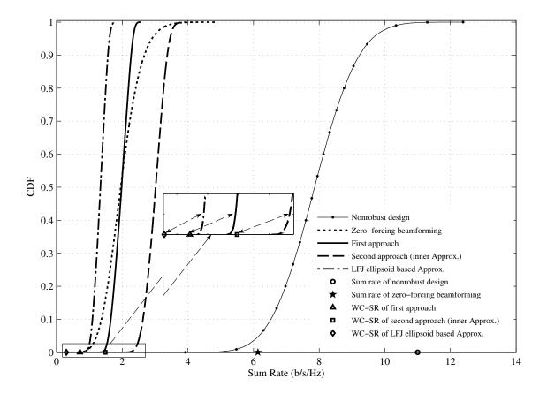
Fig. 6. CDF of the sum rate of three approaches when channel errors (for each link) are uniformly distributed in a box of size  $\rho = 0.2$  and SNR = 10 dB. The zero-forcing strategy is adopted from [3], [4].
