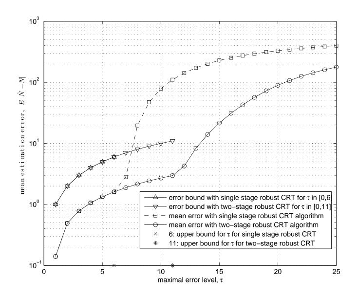
Fig. 2. Mean estimation error and theoretical error bound comparison using the single stage robust CRT and the two-stage robust CRT
