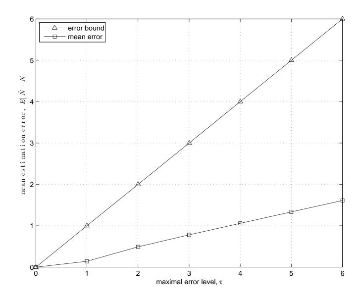
Fig. 1. Mean estimation error and theoretical error bound using the single stage robust CRT
