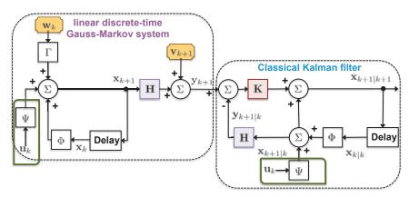
(a) Interconnection of basic state-variable system model and standard KF.
