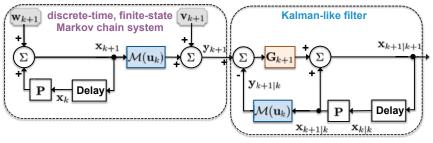
(b) Interconnection of proposed system model and Kalman-like filter
