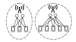
Fig. 3. The scheduling variable s is decoupled on a per-cell basis after the FP-based reformulation. Optimizing the scheduling variable s in (40) can be characterized as a weighted bipartite matching between the users and the data streams in each cell, with the matching weights defined by (44).
