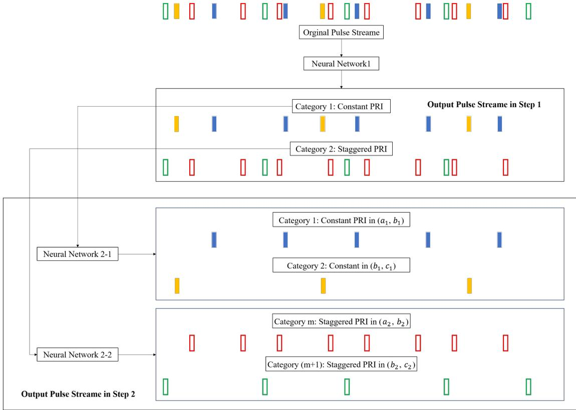
Fig. 13: Serial deinterleaving method.
