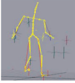
Fig. 9. Hierarchical joint skeleton.
