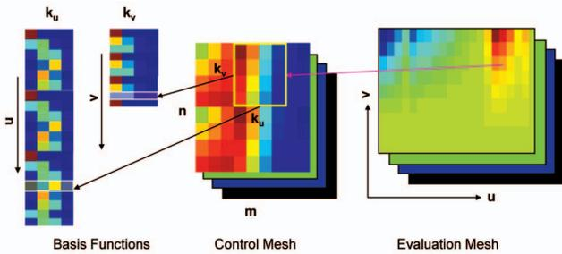
Fig. 3. Graphic showing our NURBS evaluation algorithm on the GPU. The control mesh of size  $m \times n$  and the evaluation mesh are made of four-component vectors stored as RGBA textures. The surface patch is of order  $k_u$  in the  $u$  direction and  $k_v$  in the  $v$  direction. The multiplication is restricted to the submesh of size  $k_u \times k_v$ .
