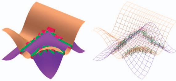
Fig. 13. Intersecting bounding boxes of two NURBS surfaces.
