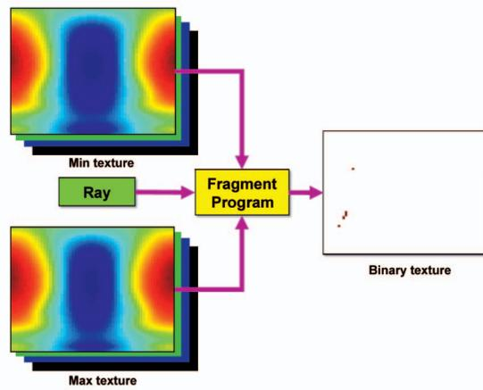
Fig. 6. Bounding-boxes stored as min and max textures are tested with the ray using a fragment program; its output is a binary texture indicating the intersection.
