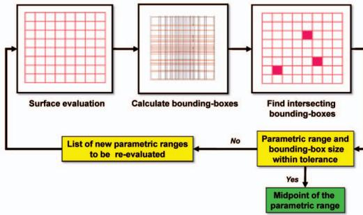
Fig. 11. Algorithm for inverse evaluation of NURBS surfaces.
