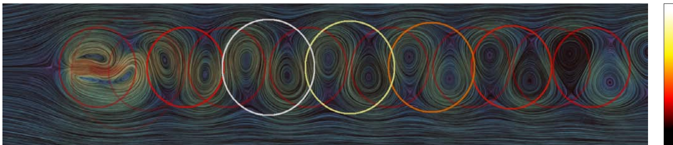
Fig. 19. For comparison, the similarity to the double vortex saddle pattern was laid over the LIC of the field with removed mean flow.
