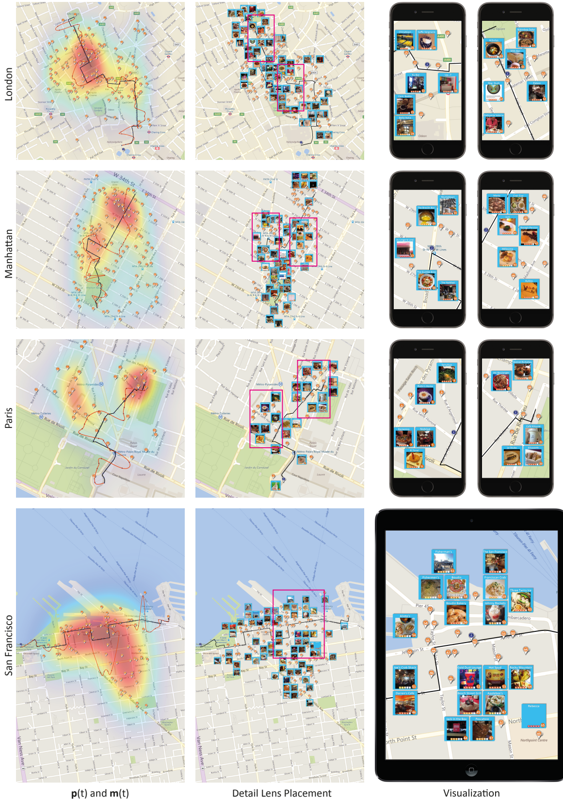
Fig. 16: Results of our framework. (left) Overview of the example areas with the queried set of POIs P and the computed paths \mathbf{p}(t) (black) and \mathbf{m}(t) (dark orange). The sum of the mixture of POI Gaussians, indicating the POI distribution, is outlined by a heat-map. (middle) The computed positions of the detail lenses. Note that the overlaps do not occur in the final visualization due to placement in different time spans. (right) Example views of the final visualization for different mobile devices (iPhone 6 Plus and iPad Air 2).
