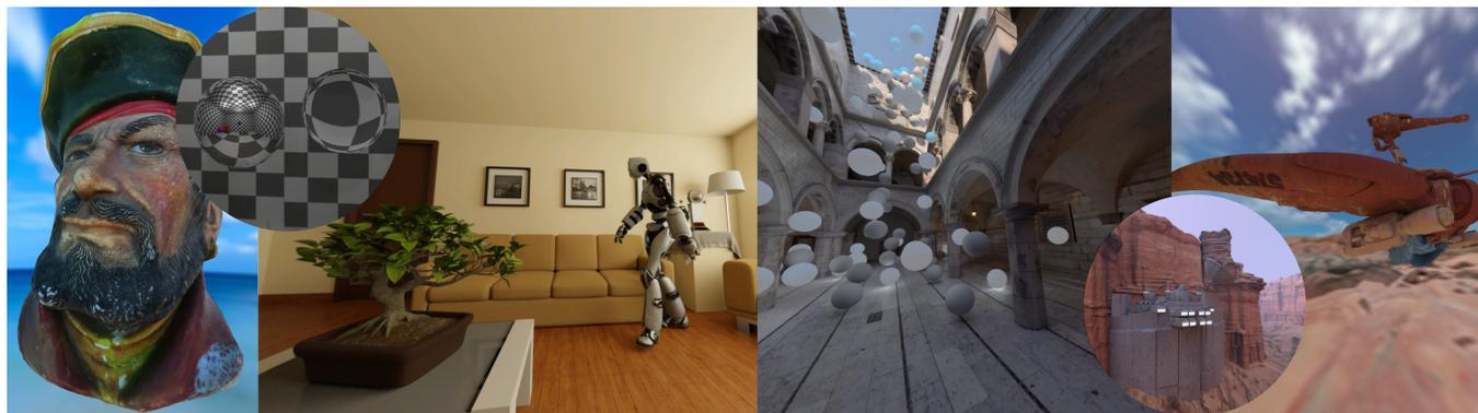
Fig. 1: Real-time ray casting reconstructions of offline-rendered animated data from a sparse set of viewpoints. Our method enables online Virtual Reality exploration of sets of pre-rendered cubemap movies with optimized placement, allowing users to experience 6 degrees of freedom with full motion parallax and view dependent lighting effects.
