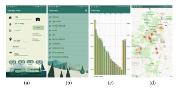
Fig. 4. The design probe's mobile application provides (a) a field notebook-style data collection interface, (b) a corresponding list of local data points collected in the field, and (c & d) interactive mobile overview visualizations based on remote server data.
