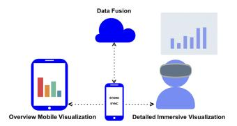
Fig. 3. An overview of our design probe architecture—data is collected and merged with cached data on a mobile device and synchronized with a cloud datastore when the device is connected. Cached data can be viewed on the mobile device or explored in a portable immersive headset.
