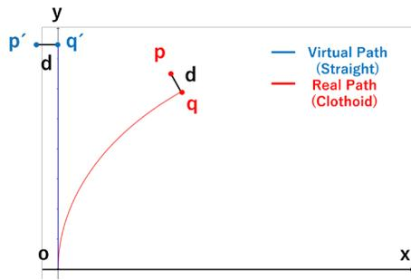
Fig. 3. An overview of the manipulation with dynamic curvature gain, showing a mapping from a clothoid path in the RE to a straight path in the VE. The user's position in RE is  $p$ , and that in VE is  $p'$ , and they are radially offset from the default path,  $q$ , in RE and  $q'$  in VE by  $d$ .
