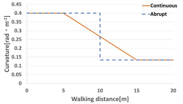
Fig. 10. Walking distance and curvature change for two forms of bending (i.e., Continuous and Abrupt) when the target gain was three. The detail for each condition is as follows: Continuous: Path condition with dynamic bending gain. 0–5 m is a no-gain section, 5–15 m is a dynamic bending gain section, and 15–20 m is a constant bending gain section and Abrupt: path condition without dynamic bending gain. 0–10 m is a no-gain section, and 10–20 m is a constant bending gain section.
