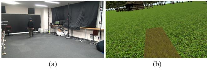
Fig. 14. Images of a scene during walking (a) Image of the RE ( $5\text{ m} \times 4\text{ m}$  tracked area). The participant walked on a clothoid path. (b) Image of the VE. The participant walked on a straight path.
