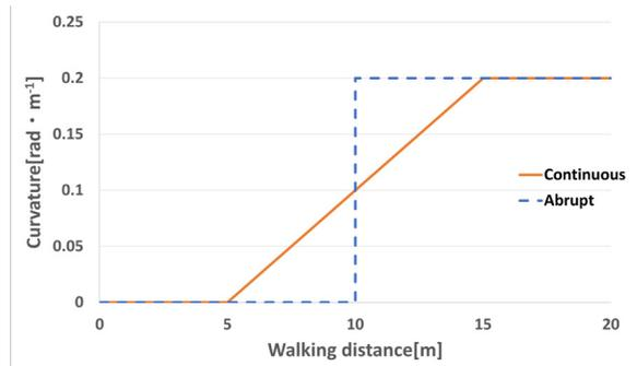
Fig. 13. Walking distance and curvature change for two forms of bending (i.e., Continuous and Abrupt) when the target gain was three. The detail for each condition is as follows: Continuous: Path condition with dynamic curvature gain. 0–5 m is a no-gain section, 5–15 m is a dynamic curvature gain section, and 15–20 m is a constant curvature gain section and Abrupt: Path condition without dynamic curvature gain. 0–10 m is a no-gain section, and 10–20 m is a constant curvature gain section.
