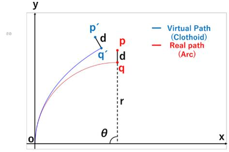
Fig. 2. An overview of manipulation with dynamic bending gain, showing a mapping from an arc path in the RE to a clothoid path in the VE. The user's position in the RE is  $p$ , and that in the VE is  $p'$ , and they are radially offset from the default path,  $q$ , in the RE and  $q'$  in the VE by  $d$ .  $r$  is the radius of the path in the RE, and  $\theta$  is the angle corresponding to the user's movement in the RE.
