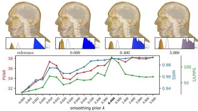
Fig. 7. Effect of the smoothing prior (Equation 12). A small value of  $\lambda$  leads to “jagged” TFs which can accurately predict small details like the teeth in blue but introduce low frequency color shifts resulting in low PSNR and SSIM [52]. A large smoothing prior smooths out small details.
