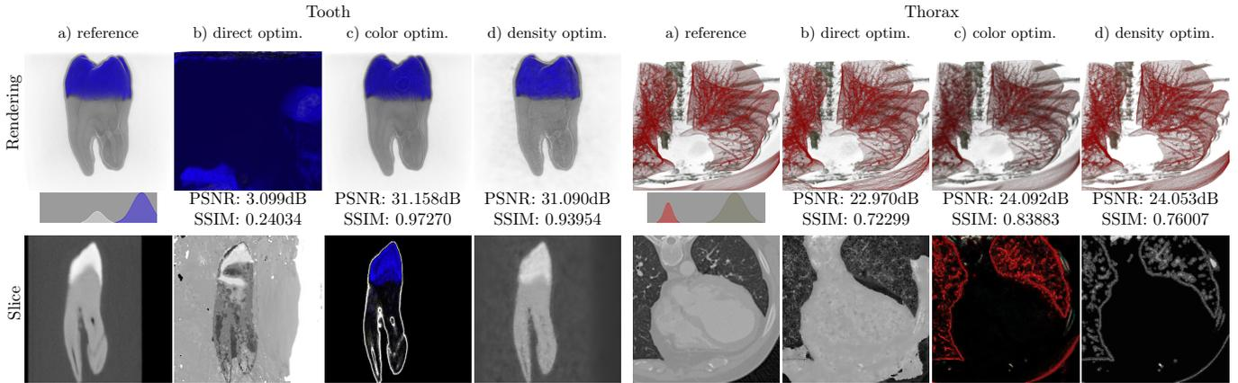
Fig. 11. Density optimization for a volume colored via a non-monotonic  $\text{rgb}\alpha\text{-TF}$  using an emission-absorption model. (a) Rendering of the reference volume of a human tooth and a human thorax. (b) Local minimum of the loss function. (c) Pre-shaded color volume as initialization. (d) Final result of the density volume optimization with TF mapping. The second row shows slices through the volumes. Note the colored slice through the pre-shaded color volume in (c).
