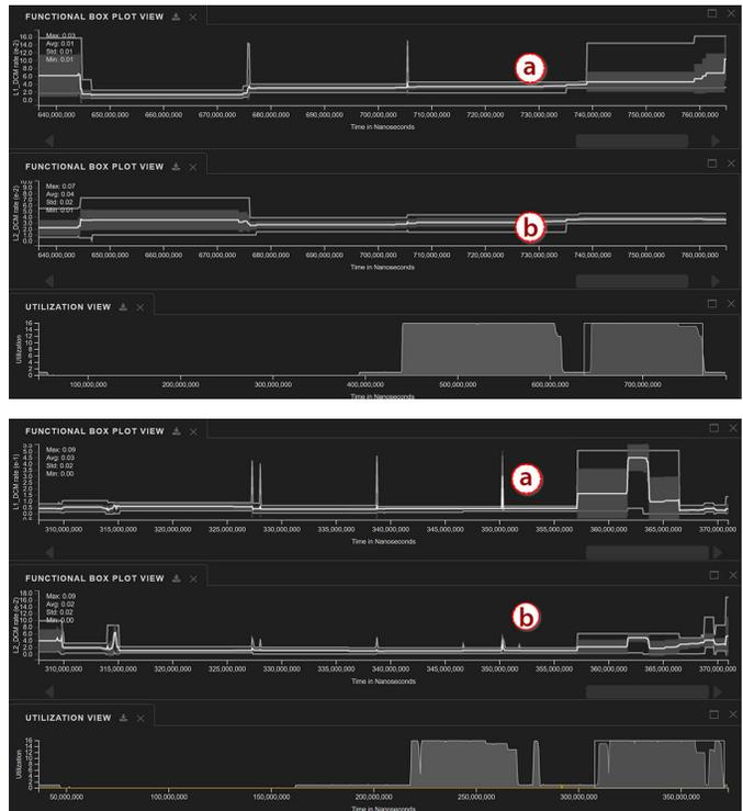
Fig. 2. Traveler helps identify cache behavior differences between Phylanx-Blaze (top) and Phylanx-Halide (bottom). The Functional Box Plots of L1 (a) and L2 (b) cache miss rates show the L2 rate rises steadily during the execution in Phylanx-Blaze while the Phylanx-Halide version remains flat.
