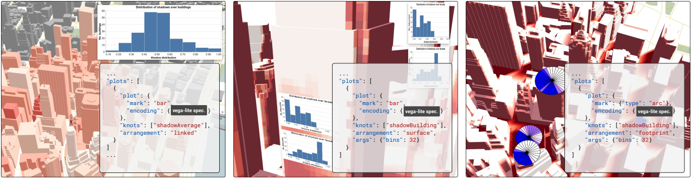
Fig. 5: Different types of physical and thematic layers integration. Left: linked view showing the distribution of sunlight access. Middle: embedded surface plots showing the distribution of sunlight access over building surfaces. Right: embedded footprint plots showing horizontal cross-section distribution of sunlight access.
