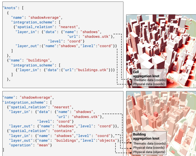
Fig. 4: UTK abstracts spatial joins through the use of knots . Top: Knot integrating thematic and physical layers. Bottom: Knot integrating a thematic layer with the average per building.
