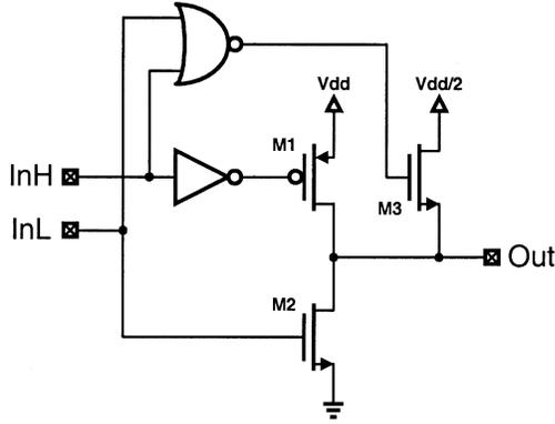
Fig. 3. ATLS system transmitter.
