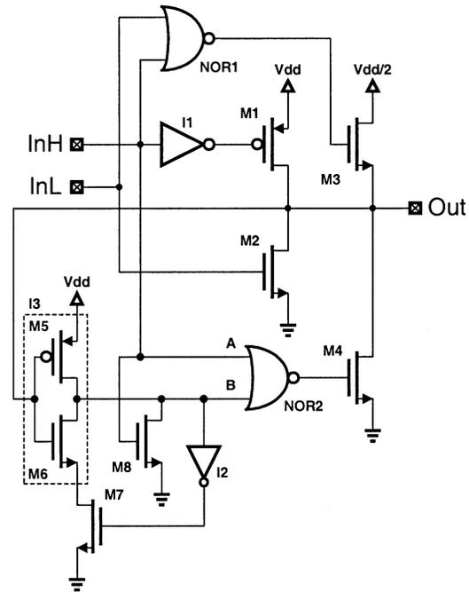
Fig. 6. Enhanced ATLS system transmitter.
