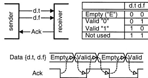
Fig. 1. Dual-rail four-phase protocol.
