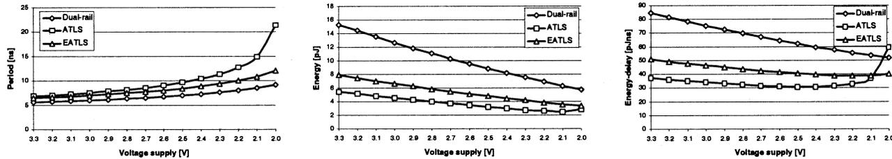
Fig. 9. Period, energy, and energy-delay product versus supply voltage at 10-mm-wire length.
