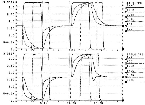
Fig. 4. Output waveforms of basic (upper graph) and enhanced (lower graph) ATLS system.
