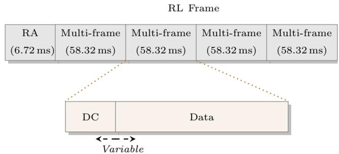
Fig. 1: Framing structure of LDACS RL communication.
