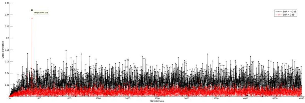
Fig. 8: Correlator output at SNR of 0dB and  $-10$ dB.
