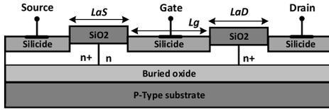
Fig. 4. Schematic cross section of the SOI MEFET [14].
