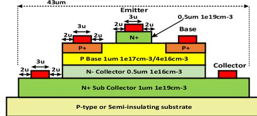
Fig. 9. Cross-sectional schematic of 4H-SiC BJT device topology [30].
