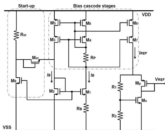
Fig. 1. CMOS SOI-based voltage reference circuit [11].
