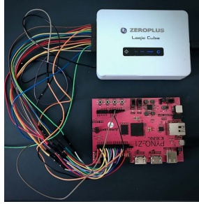
Fig. 5. Measurement setup with logic analyzer.
