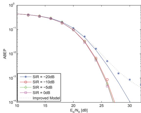
Fig. 10. ABEP of the  $T_c$ -DTR receiver with 3 interferers located at  $f_{J_1} = 0.9054\text{GHz}$  (GSM band),  $f_{J_2} = 1.38105\text{GHz}$  (GNSS band), and  $f_{J_3} = 2.452\text{GHz}$  (802.11b Wi-Fi band). The “Improved Model” is given in Section IV-B. The receiver is optimized (on average) to reject the aggregate NBI (see (28)): i)  $C_1 = 0$ , ii)  $\sum_{j=1}^{N_s-1} c_j c_{j-1} = -31$ , and iii)  $T_c = 75.65\text{ns}$ .
