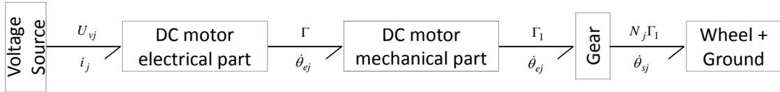
**Figure 4.4:** Word bond graph of a quarter RobuTAINeRs (electromechanical subsystem).
