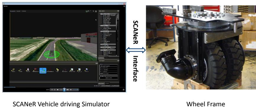
**Figure 4.10:** *SCANeR Studio* driving simulator and the wheel frame of RobuTAINeR that was modeled with *Matlab/Simulink*.
