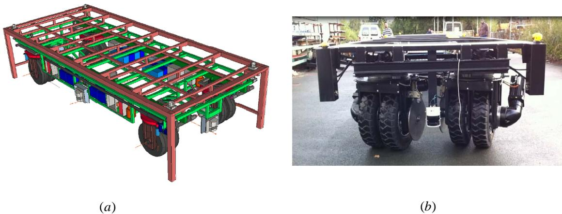
**Figure 4.2:** (a) CAD figure of RobuTAINeR's prototype, (b) Real RobuTAINeR picture.
