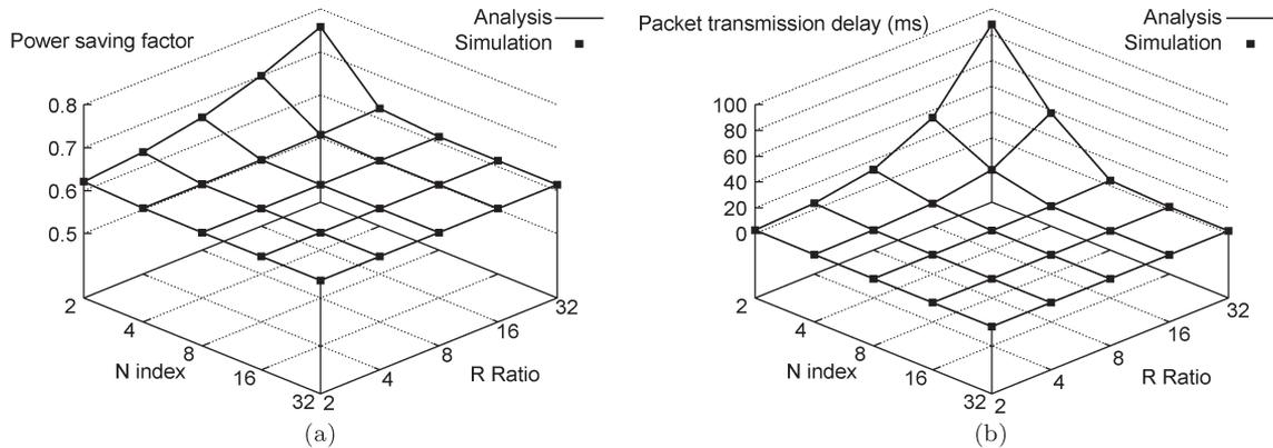
Fig. 4. Power-saving factor and average packet transmission delay when  $\tau = 0.1$  ms,  $\lambda = 0.1/\text{ms}$ ,  $C_S = 8$  ms, and  $C_T = 8$  ms. (a) Power-saving factor. (b) Average packet transmission delay.
