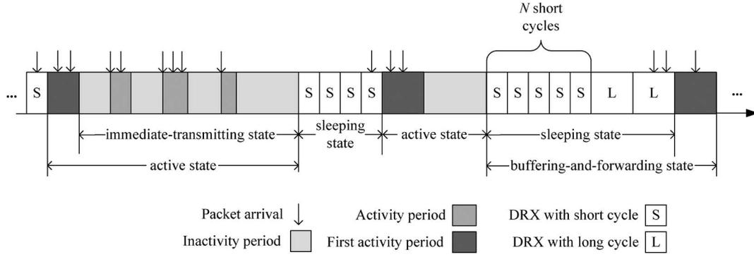
Fig. 1. Exemplary snapshot of the DRX operation in 3GPP LTE Advanced wireless networks.
