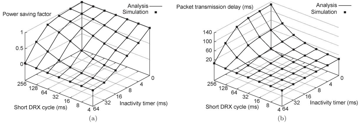
Fig. 3. Power-saving factor and average packet transmission delay when  $N = 2$ ,  $\tau = 0.1$ ,  $\lambda = 0.1$ , and  $C_L = 2C_S$ . (a) Power-saving factor. (b) Average packet transmission delay.
