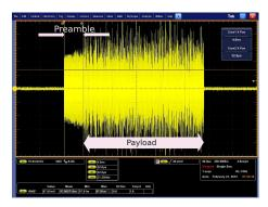
Fig. 11. Transmitted 802.11p frame captured by the spectrum analyzer. The representation in the time domain shows that the preamble features stable power levels, while the OFDM signal (i.e., PLCP, MAC, and WSMP headers, as well as payload) exhibits irregular power patterns.
