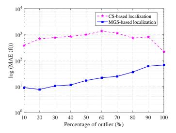
Fig. 8. The MAE for MGS-based and CS-based localization schemes with an increasing rate of APs that contain outlier. The MGS-based localization is robust to the outliers while the CS-based localization show very large localization errors even with a low percentage of outliers.
