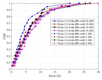
Fig. 12. The cumulative distribution of the localization error when  $\frac{1}{2}$ ,  $\frac{1}{3}$ ,  $\frac{1}{4}$ ,  $\frac{1}{5}$  of the RPs are used for radio map interpolation when 5 and 19 APs are used for localization.
