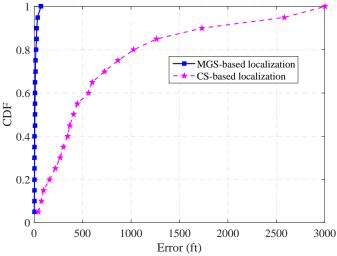
Fig. 9. The cumulative distribution localization error for MGS-based and CS-based localization schemes. The CS-based localization error are inordinate showing the sensitivity of the approach to the system malfunctioning. The MGS-based localization shows a great low distribution of errors.
