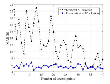
Fig. 5. The MAE for GS-based localization using the two different AP selection schemes: Strongest AP and Fisher Criteron.
