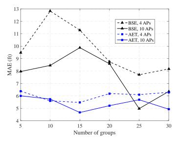
Fig. 11. The average localization error versus different number of groups for two different environments when 4 and 10 APs are used.
