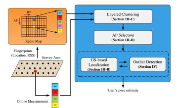
Fig. 1. The schematic of the proposed scheme.
