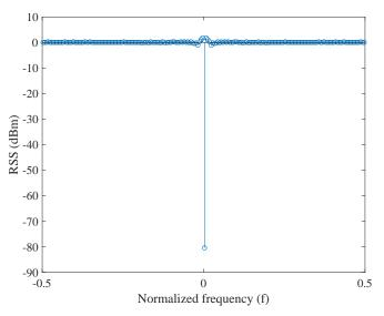
Fig. 3. The frequency representation of the RSS fingerprints for an AP. The great sparse profile shows the potential for RSS interpolation using the sparse recover algorithm.
