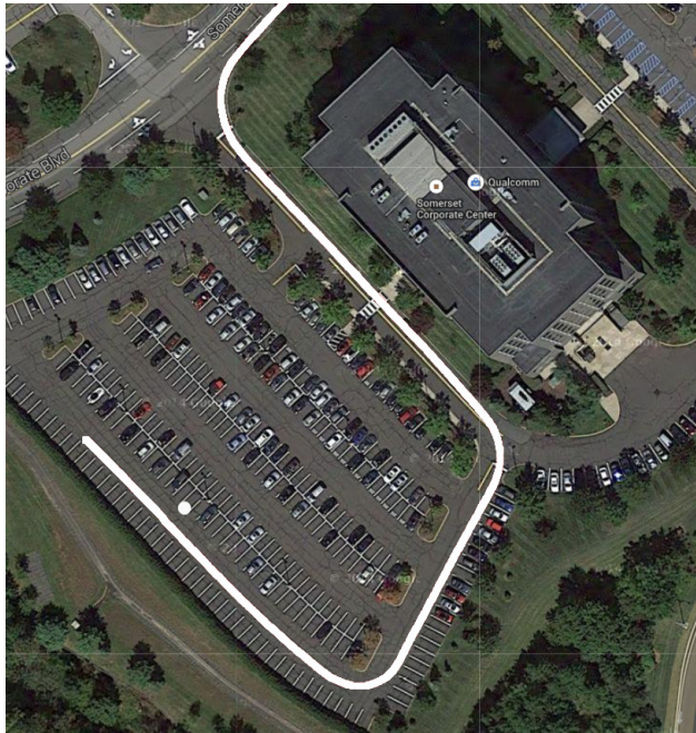
Fig. 8. Vehicle trajectory (directed from left to top) plotted on Google Maps. The white dot indicates the position of the static MDP.
