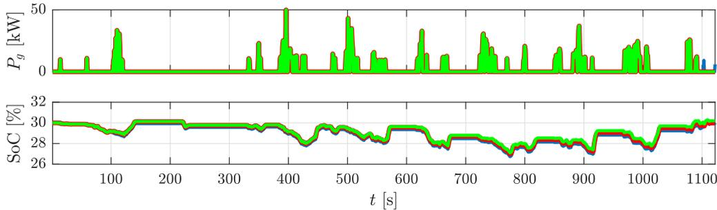
Figure 7: DP (blue), PMP (red) and analytical method (green) results. The upper plot corresponds to the control action,  $P_g$ , and the bottom plot to the state, battery SoC
