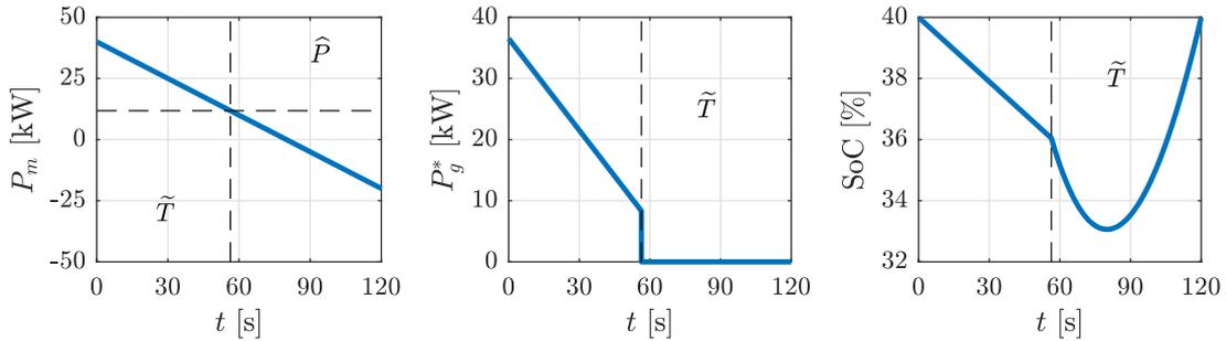
Figure 5: Trajectory and optimization solution for an example case of 120 seconds. The left plot shows the  $P_m$  trajectory, the middle plot shows the optimized generator set power output, and the right plot shows the variations on battery’s SoC throughout the example with an initial level of 40%.
