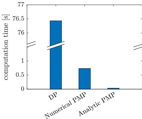
Figure 9: Computation time of optimization methods at the example driving cycle.
