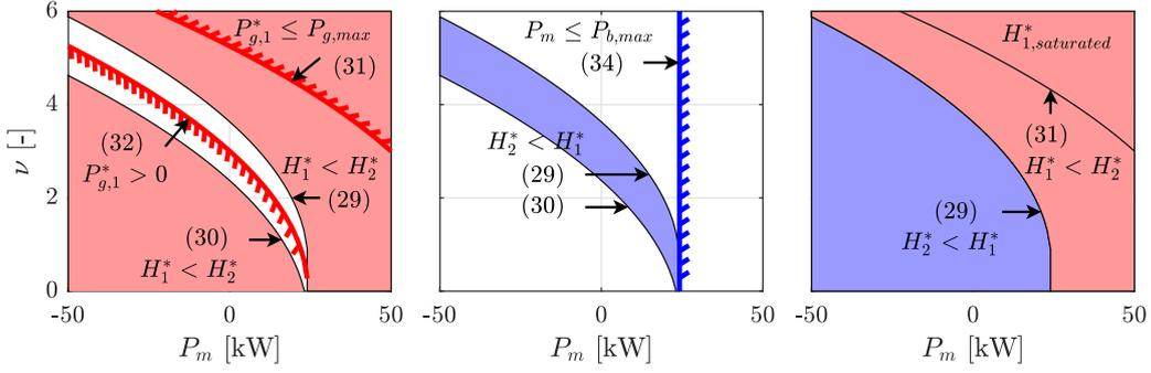
Figure 3: Graphical representation of both candidates for minimum,  $H_1^*$  (left) and  $H_2^*$  (center). Solid colors represent regions where one candidate is the minimum; hatched lines represent constraints (corresponding equations are indicated). Combining both candidates and constraints results in the right plot where active regions are shown for  $H_1^*$  (red) and  $H_2^*$  (blue).
