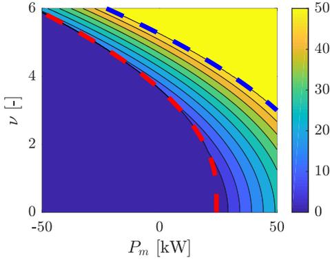
Figure 4: Representation of optimal set of actuations  $P_g^*$  for different levels of traction requirements ( $P_m$ ) and parameter  $\nu$ . The red dashed line is the generator set disconnection limit, (37), and the blue dashed line is the generator set maximum power constraint, (33).
