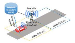
Fig. 2. Road map information exchange among an intelligent vehicle, a roadside unit, and the map data repository in a V2X network.
