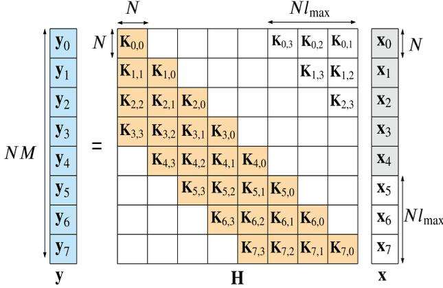
Fig. 2. The delay-Doppler domain input-output relation  $\mathbf{y} = \mathbf{H} \cdot \mathbf{x}$  after adding null symbols only contains the shaded blocks for  $N = M = 8$  and  $l_{\max} = 3$ .
