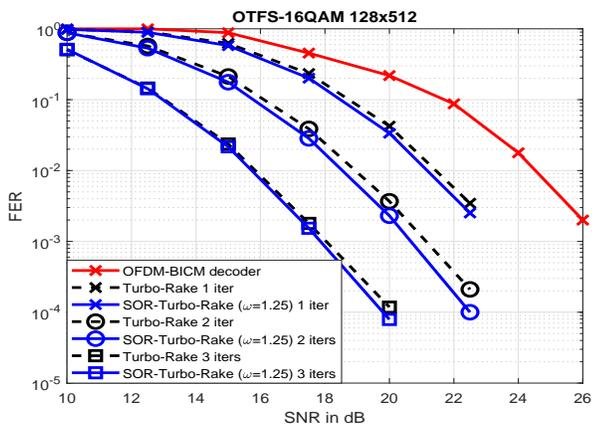
Fig. 11. Turbo 16-QAM FER Plot: MRC vs BIC-MMSE-OFDM.
