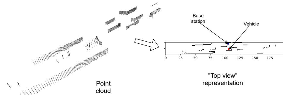
Fig. 1: Preprocessing of the LIDAR point cloud.
