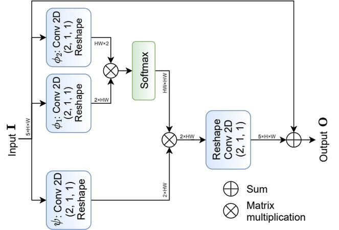
Fig. 3: Block diagram of the non-local attention module.
