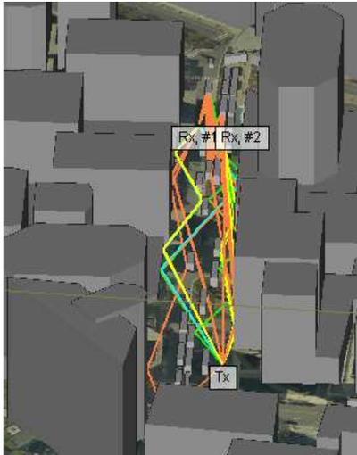
Fig. 7: Four-lane road simulation in an urban canyon scenario.
