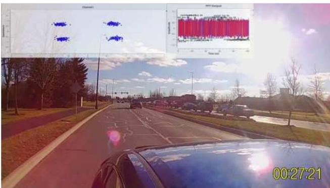
Fig. 16: SPaT messages collected from a moving vehicle. The received signal and the constellation diagram are seen at the upper left.
