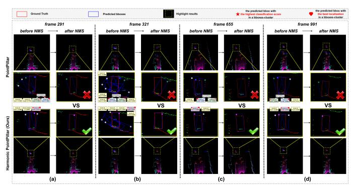
Fig. 5. Qualitative analysis of inconsistent/consistent 3D detection. For better view, the results are in BEV visualization (zoom in for detail check). PointPillar (baseline) [21] suffers from inconsistency problem in 3D detection, while Harmonic PointPillar (Ours) shows a great robustness on keeping predictions consistent.
