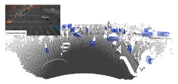
Fig. 6. Qualitative example of on-infrastructure LiDAR-based 3D object detection (detection results (blue bboxes) are made by our proposed method: Harmonic PointPillar).
