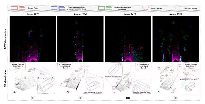
Fig. 4. Qualitative analysis of overall 3D detection performance. Predicted bboxes from Pointpillar (baseline) (green bboxes) [21] and predicted bboxes from Harmonic Pointpillar (Ours) (blue bboxes) are visualized in same frames. Ground Truths (red bboxes) are also drawn for qualitative check. Harmonic PointPillar (Ours) shows better recall rate and localization accuracy with less false positive than PointPillar (baseline).
