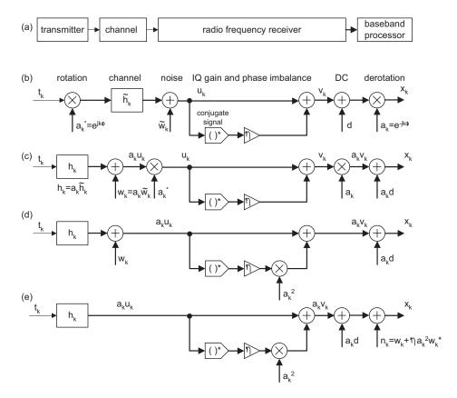
Fig. 1. Block diagram to derive the signal model.
