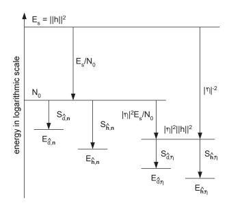
Fig. 2. Level diagram to explain the contribution of the different error and suppression terms.
