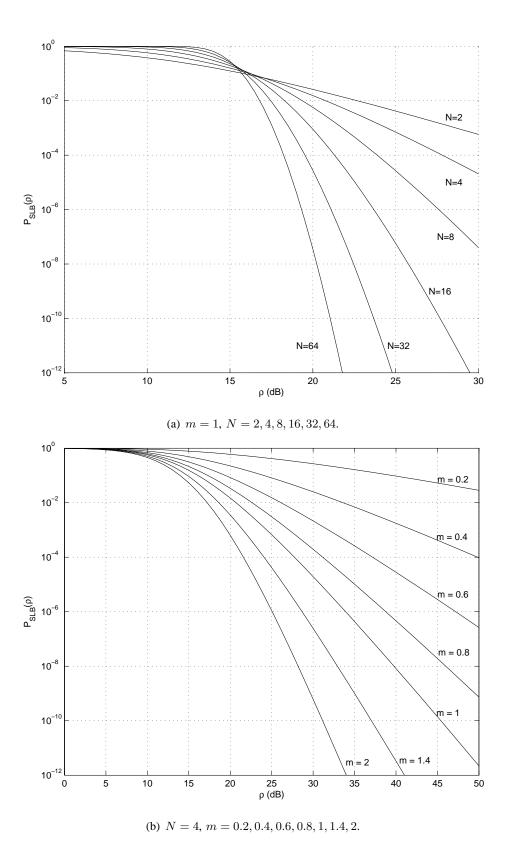
Fig. 2. Sphere lower bound  $P_{\rm slb}(\rho)$  for various values of N and m.
