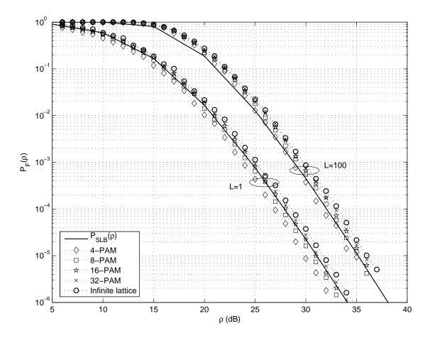
Fig. 9. Frame error probability  $P_{\rm f}(\rho)$  of the finite constellation generated with 4,8,16,32-PAM,  $P_{\rm f}(\rho)$  with N=4 of the infinite lattice and sphere lower bound  $P_{\rm slb}(\rho)$  for L=1,100 with the Krüskemper rotation.
