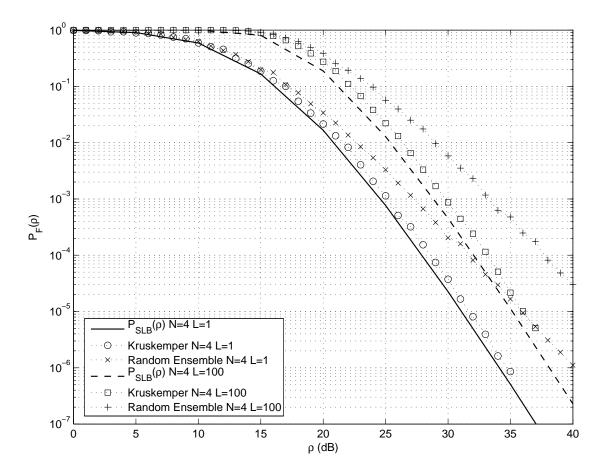
Fig. 6. Frame error probability  $P_{\rm f}(\rho)$  and sphere lower bound  $P_{\rm slb}(\rho)$  for m=1,~N=4,~L=1,100 with Krüskemper rotation.
