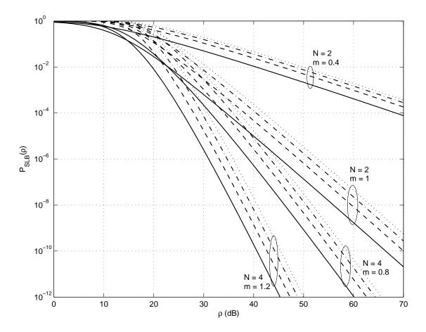
Fig. 3. Sphere lower bound  $P_{\rm slb}(\rho)$  for L=1 (solid), L=10 (dashed), L=100 (dashed-dotted) and L=1000 (dotted) and various values of N and m.
