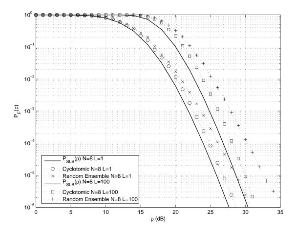
Fig. 7. Frame error probability  $P_{\rm f}(\rho)$  and sphere lower bound  $P_{\rm slb}(\rho)$  for  $m=1,\,N=8,\,L=1,100$  with cyclotomic rotation.
