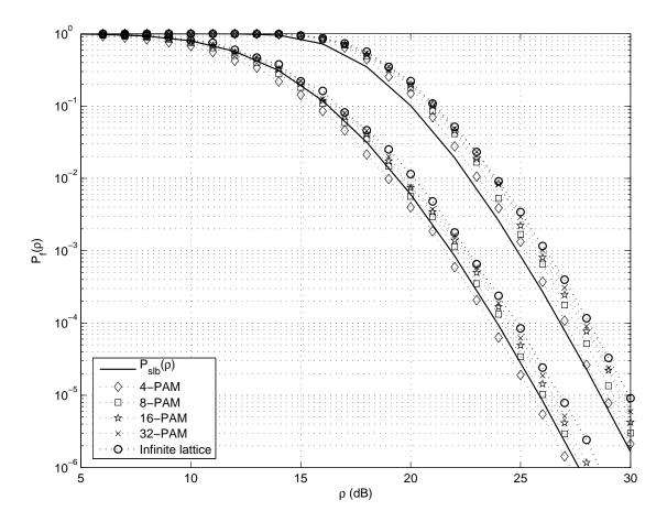
Fig. 10. Frame error probability  $P_{\rm f}(\rho)$  of the finite constellation generated with 4,8,16,32-PAM,  $P_{\rm f}(\rho)$  with N=8 of the infinite lattice and sphere lower bound  $P_{\rm slb}(\rho)$  for L=1,100 with the cyclotomic rotation.
