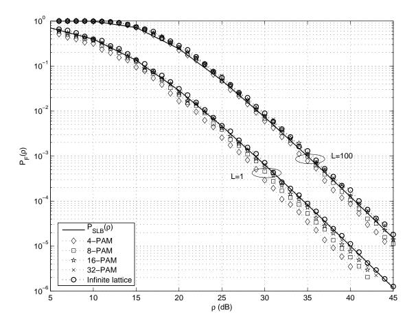
Fig. 8. Frame error probability  $P_{\rm f}(\rho)$  of the finite constellation generated with 4,8,16,32-PAM,  $P_{\rm f}(\rho)$  with N=2 of the infinite lattice and sphere lower bound  $P_{\rm slb}(\rho)$  for L=1,100 with the cyclotomic rotation.
