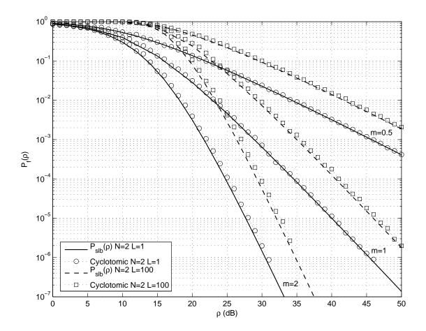
Fig. 4. Frame error probability  $P_{\rm f}(\rho)$  and sphere lower bound  $P_{\rm slb}(\rho)$  for  $N=2,\,m=0.5,1,2$  and L=1,100.
