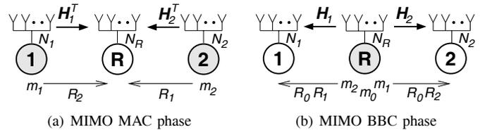
Fig. 1. Decode-and-forward bidirectional relaying with multiple antennas at all nodes. In the initial multiple access (MAC) phase, nodes 1 and 2 transmit their messages  $m_1$  and  $m_2$  with rates  $R_2$  and  $R_1$  to the relay node. In the succeeding bidirectional broadcast (BBC) phase, the relay forwards the messages  $m_1$  and  $m_2$  with rates  $R_2$  and  $R_1$  and adds its own common message  $m_0$  with rate  $R_0$  to the communication.
