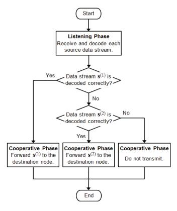
Fig. 4. Flow chart of the processing at the relay node. The source node sends two independent data streams to the destination node. The relay node attempts to decode and forward one data stream to the destination node.
