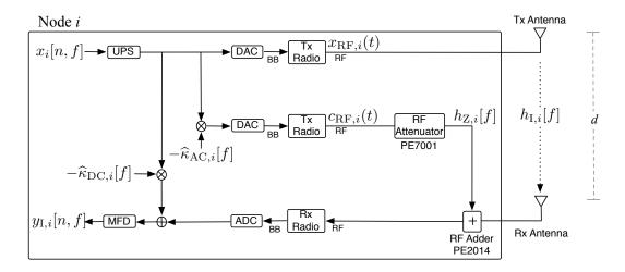
Fig. 1. Block diagram of a full-duplex node.
