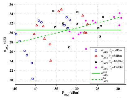
(a) Results for active analog cancellation. The constant fit is equal to  $\alpha_{{\rm AC},i}^{{\rm con}}=30.55~{\rm dB}$  and the linear fit is equal to  $\alpha_{{\rm AC},i}^{{\rm lin}}=\lambda_{{\rm AC}}{\rm P}_{{\rm RI},i}+\beta_{{\rm AC}}$  where  $\lambda_{{\rm AC}}=0.21~{\rm dB/dBm}$  and  $\beta_{{\rm AC}}=37.42~{\rm dB}$ .
