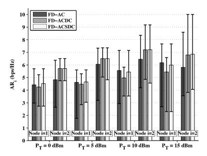
Fig. 11. Experiment results showing the effect of different cancellation schemes on the achievable rate per node of a full-duplex two-way system using the same transmission power  $P_T$  at both nodes. Results correspond to d=20 cm and a distance between Node 1 and Node 2 equal to 8.5 m. Each bar corresponds to results from two 800 frame experiments.
