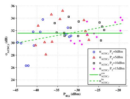
(b) Results for combined active analog and active digital cancellation. The constant fit is equal to  $\alpha_{\text{ACDC},i}^{\text{con}}=31.56$  dB and the linear fit is equal to  $\alpha_{\text{ACDC},i}^{\text{lin}}=\lambda_{\text{ACDC}}P_{\text{RI},i}+\beta_{\text{ACDC}}$  where  $\lambda_{\text{ACDC}}=0.12$  dB/dBm and  $\beta_{\text{AC}}=35.49$  dB.
