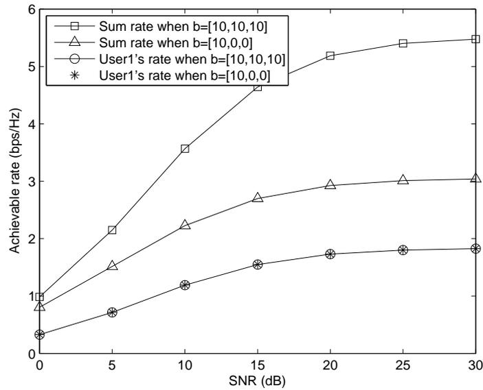
Fig. 2. The sum rate and the achievable rate at the user 1 in  $3 \times 3$  MIMO BC. The achievable rate of user 1 is not affected by the other users' feedback sizes, while the sum rate is increased as the feedback sizes of other users increase.
