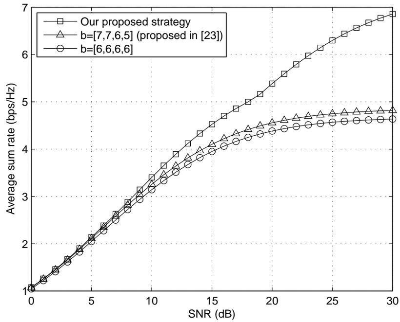
Fig. 4. Sum rates of a  $4 \times 4$  MIMO BC using various feedback rate sharing strategies ( $\sum b_k = 24$ ). Different path losses among the users are considered  $(\gamma_1, \gamma_2, \gamma_3, \gamma_4) = (1.5, 1.25, 1, 0.75)$ .
