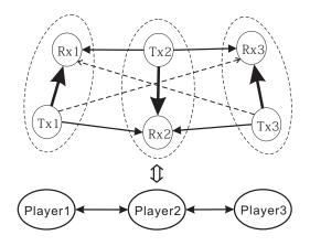
Fig. 1. The chain-like topology for 3 transmit-receive pairs
