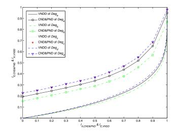
Fig. 7: EXIT chart for different degree distributions
