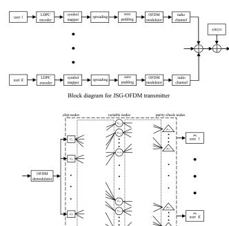
Block diagram for JSG-OFDM receiver
