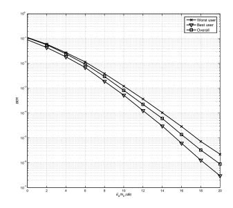
Fig. 13: Performance of different users in JSG-OFDM
