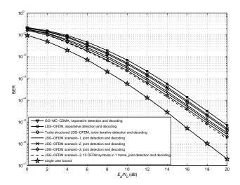
Fig. 10: Performance of 300% loaded systems over ITU Pedestrian Channel B
