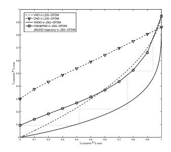
Fig. 4: EXIT chart over AWGN Channel at  $E_b/N_0 = 9$  dB
