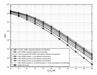
Fig. 9: Performance of 200% loaded systems over ITU Pedestrian Channel B
