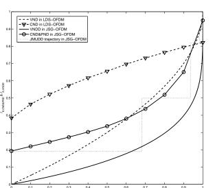
Fig. 5: EXIT chart over ITU Pedestrian Channel B at  $E_b/N_0$  = 13 dB
