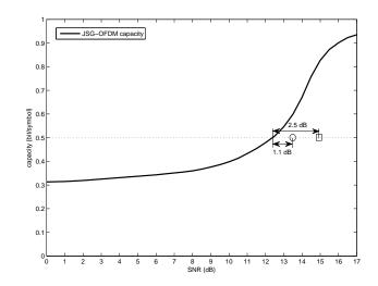
Fig. 11: Maximum effective throughput of JSG-OFDM over ITU Pedestrian Channel B
