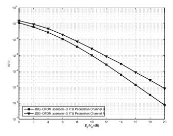
Fig. 15: Performance of JSG-OFDM over different multipath channels
