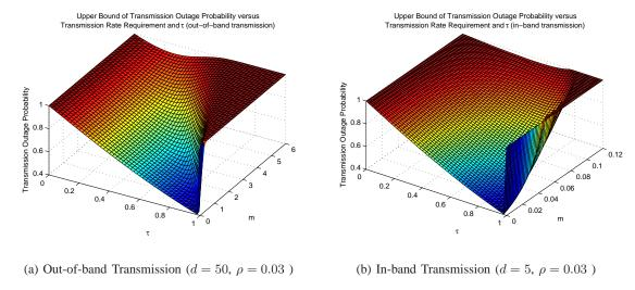
Fig. 13. Upper bound of transmission outage probability versus transmission rate requirement and  $\tau$  (time-switching architecture).
