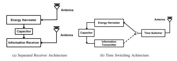
Fig. 2. Separated receiver and time switching architectures.
