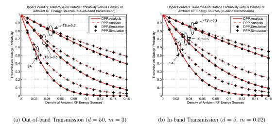
Fig. 10. Upper bound of transmission outage probability versus density of ambient RF energy sources.
