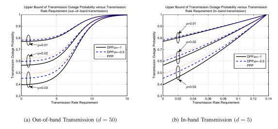
Fig. 12. Upper bound of transmission outage probability versus transmission rate requirement (separated receiver architecture).
