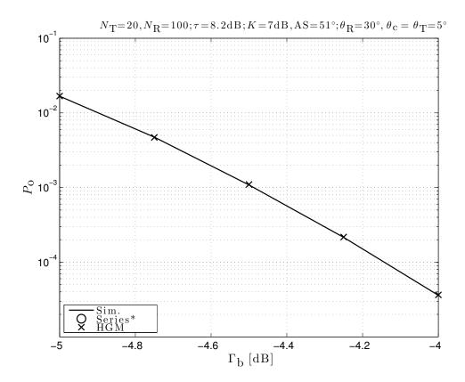
Fig. 3. Stream-1 outage probability for  $N_R = 100$ ,  $N_T = 20$ , for K = 7 dB and AS =  $51^{\circ}$  (i.e., averages for scenario A1). Results corresponding to Series do not appear because of numerical divergence.
