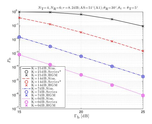
Fig. 1. Stream-1 outage probability for  $N_R = 6$ ,  $N_T = 4$ ,  $AS = 51^{\circ}$  (i.e., scenario A1 mean), and various values of K, including K = 7 dB (i.e., scenario A1 mean). Series results for K = 14,21 dB do not appear because of numerical divergence.
