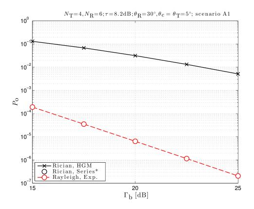
Fig. 2. Stream-1 outage probability for  $N_R = 6$ ,  $N_T = 4$ , averaged also over the WINNER II lognormal distributions of K and AS for scenario A1. Results corresponding to Rician, Series do not appear because of numerical divergence.
